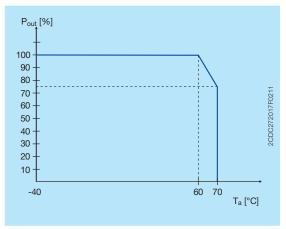
Characteristic curve of temperature at rated load
