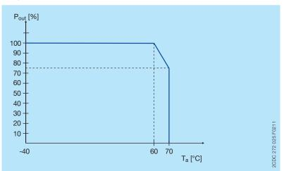
Characteristic curve of temperature at rated load
